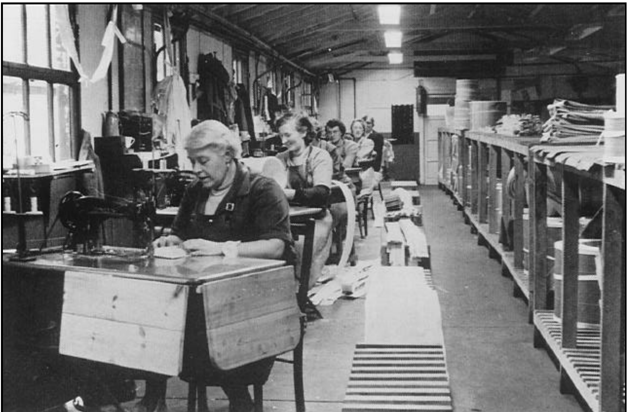
32. Machinists at Vokes at Henley Park making filters out of gauze and steel mesh in the early 1950s.
